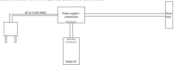
! Note: The relay switch of the Robin doesn't supply power for the electronic lock! Make sure that the switched voltage does not exceed 48V and the switched power is max. 12W. !
