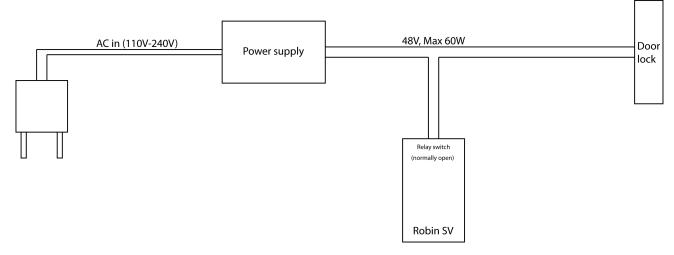
Electronic door lock with input contact on the control box:
