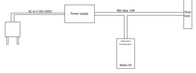
Electronic door lock with input contact on the control box:
