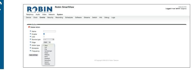
The green '+' creates a new 'Action'. The '>>' behind a line opens the details for this 'Action'. The red X behind a line deletes the 'Action' from the list.
