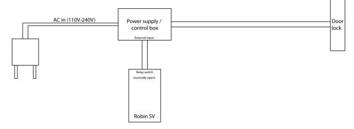
! Note: The relay switch of the Robin doesn't supply power for the electronic lock! Make sure that the switched voltage does not exceed 48V and the switched power is max. 12W. !
